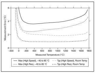
Figure 10. Thermocouple Types R and S Errors
