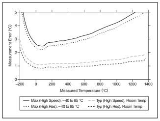
Figure 7. Thermocouple Type K Errors
