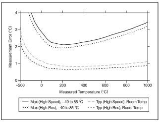
Figure 8. Thermocouple Types T and E Errors
