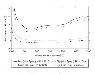
Figure 6. Thermocouple Types J and N Errors
