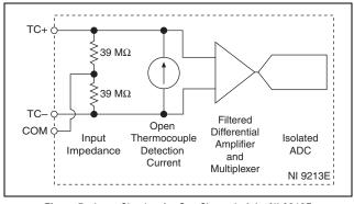
Figure 5. Input Circuitry for One Channel of the NI 9213E
