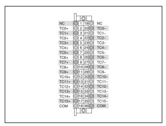
Figure 2. NI 9213E Terminal Assignments
