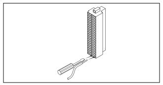
Figure 4. Connecting Wires to the NI 9213E Connector
