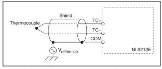
Figure 3. Connecting a Shielded Thermocouple Input Signal to the NI 9213E
