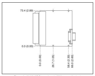
Figure 1. NI 9213E Dimensions in Millimeters (Inches)
