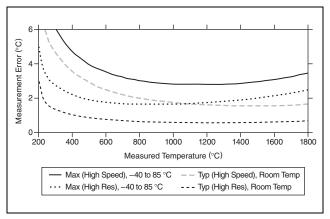
Figure 9. Thermocouple Type B Errors
